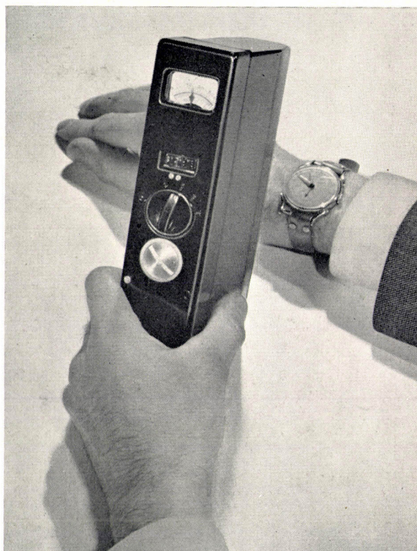
Fig. 9. The Geiger counter in use. The illustration reveals the fact that the very weak radio-active radiations from the luminous dial of a wrist watch can be registered.
