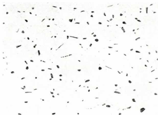
Fig. 6. An etched section through an internally oxidized Cu-Zn alloy (99% Cu-1% Zn) clearly shows oxide particles, when enlarged 500 times. The material was heated for 3\frac{1}{2} hours at 950 °C in air.
