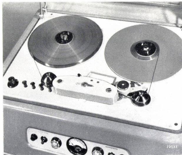
Fig. 7. Close-up of the top panel of the magnetic recorder depicted in fig. 6 . The components of the driving mechanism sketched in fig. 1 are easily recognized. At the front of this panel, on the left, will be seen the push-buttons for the control. The first of these (left to right) is for the rewind; rotation of the knob on the extreme left controls the speed, both forward and reverse. The second button starts the recorder at normal speed forward; this is the "playback" setting, seeing that the playback head is permanently connected to the amplifier (all amplifiers are of course previously switched on). The third push-button brings in the erasing head and recording head. To avoid the possibility of erasing part of a recording by depressing the button accidentally, this button is interlocked in such a way that it functions only when depressed together with the second button (which merely starts the machine). The fourth button returns all the others to neutral and stops the instrument by braking the motors.
